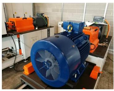
Low and Medium Voltage Motors can be tested at our premises up to 160kW
